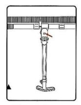
Twist open the screw and pull it out
