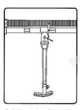
▲ Pull out the plug and remove the bracket
